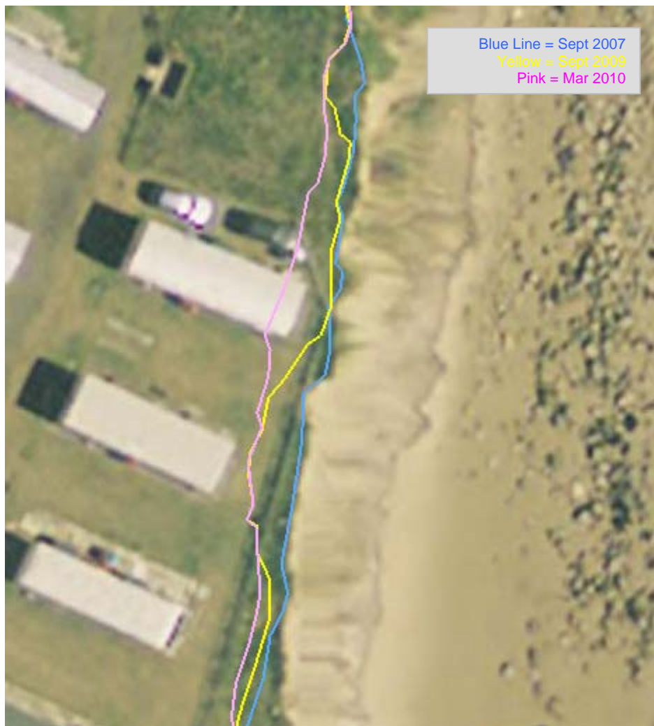
Figure 30 - Cliff Top Recession at Sandy Bay Caravan Park
